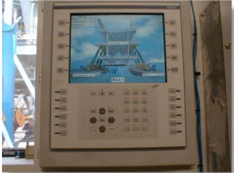
The Magelis™ interface on board a Versatruss lifting barge.
